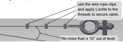
Figure 6. Restraining cable angle tolerance.
