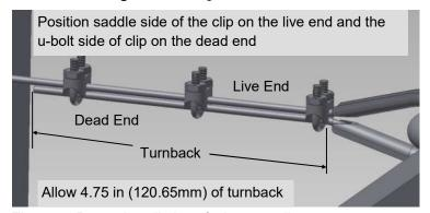
Figure 5. Proper installation of wire rope clips.
