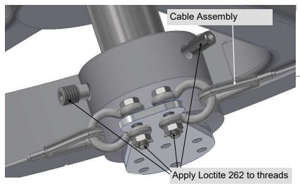
Figure 3. Installation of set screws and shackle.
