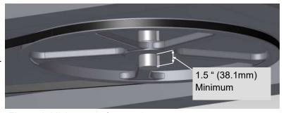
Figure 1. Minimum shaft extension.
