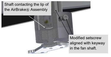
Figure 2. AirBrake® coming into contact with shaft.
