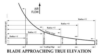
The hub serves two major (aerodynamic) purposes. It allows termination of the blades at a point where they would cease to function efficiently and it prevents back flow of air through the center.
