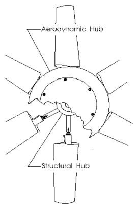
Reference to the drawing at left will readily show the necessity of a hub of some proportion. As the centerline of the wheel is approached, the chord of the blade becomes infinite. For practical reasons, it is evident that the hub in this example should start at
