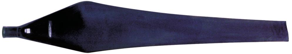
Tuf-Lite® is a single piece, hollow and light weight blade constructed from fiberglass reinforced epoxy resin. The uniqueness of a Fiberglass Reinforced Plastic (FRP) mold construction method allows the blades to be formed in an efficient airfoil shape with a gradual transition in the angle of attack, blade width, and thickness. Standard sizes are available from 5–40 feet in diameter.
