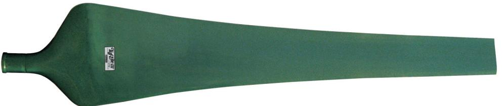
Tuf-Lite III® is a refined and enhanced one-piece blade constructed from fiberglass reinforced vinyl ester resin coupled with leading and trailing edge protection, and superior "UV" protection. Developed from the most severe strength-testing program to date, Tuf-Lite III® blades are individually balanced, interchangeable and will install in HUDSON hub designs Initial size are from 28 feet to 10 meters in diameter.
