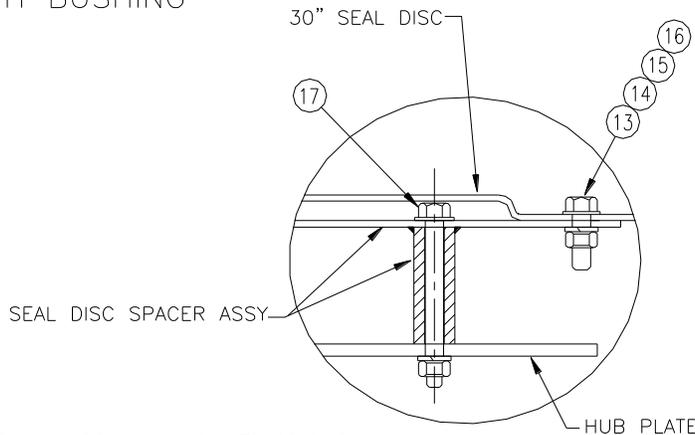
Seal Disc Spacer Mounting for 5H Hub Assy
