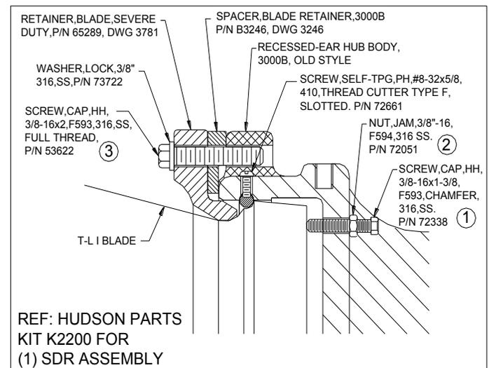
Figure 10C (old style hub & retro-fit SDR)
